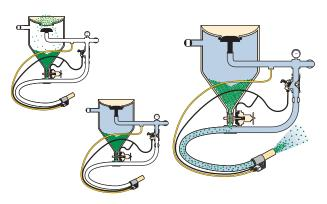
**780** (pot-under-pressure) controls, used with Empire's SuperBlast, PRS and FaStrip systems, stop blasting when the "on/off" trigger is released while maintaining pressure in the vessel. This arrangement, which conserves compressed air and is easiest on system components, is especially useful for spot blasting because of the fast restarts it provides.
