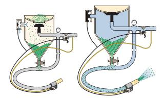
**680 (blow-down) controls**, used on SuperBlast and Econ-O-Blast™ portables, vent pressure from the vessel when the "on/off" trigger is released. This setup makes blasting easier for a single operator and permits automatic grit refills.
